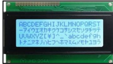
Gambar 4. LCD Dot-Matrix HD44780
