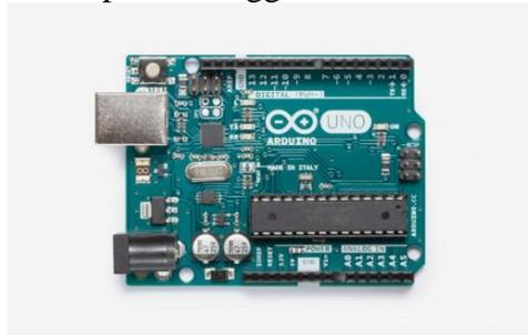
**Gambar 6.** Board Arduino Uno
